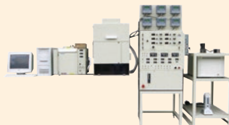
Gas permeation tester for solid polymer electrolyte membrane
