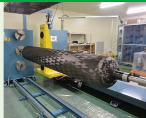
Composite cascade cylinders for hydrogen stations.
